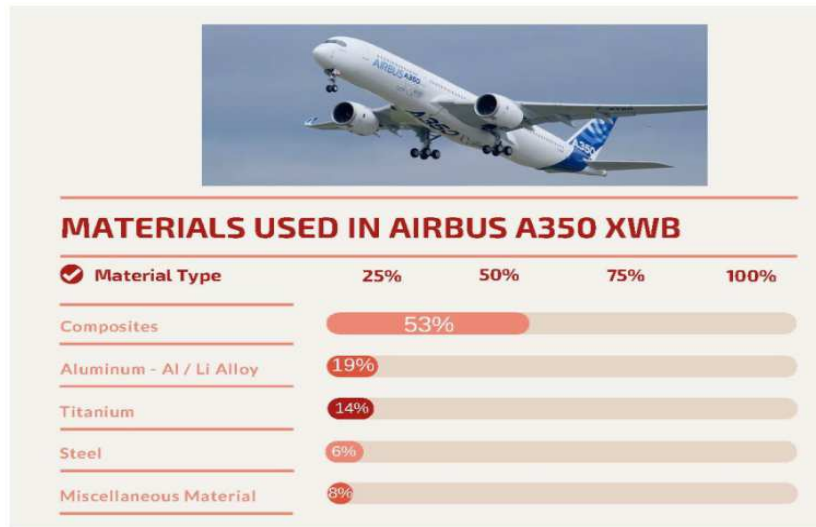
Figure 6: Materials used in Airbus A350 XWB (A. Katunin, 2016).
